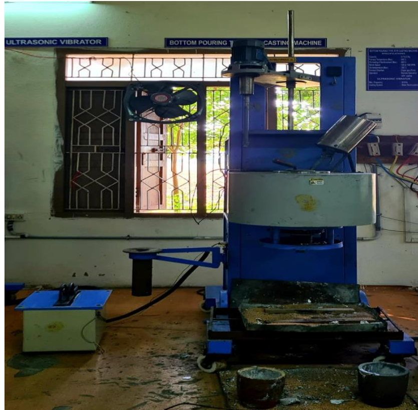
Figure 4.1 Stir Casting Setup
